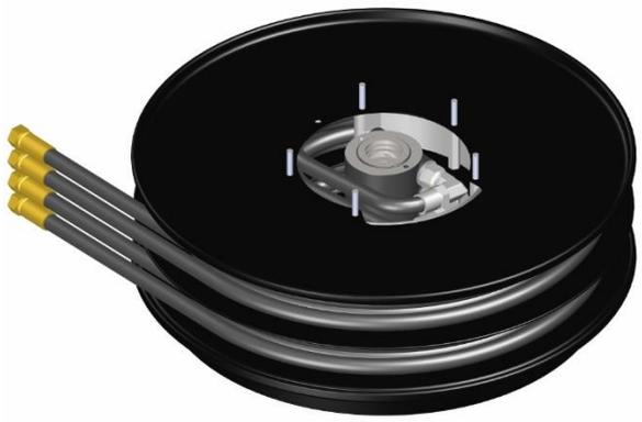
11- Unthread the whole reel body as shown in the picture, turn it over and place it on a workbench.
