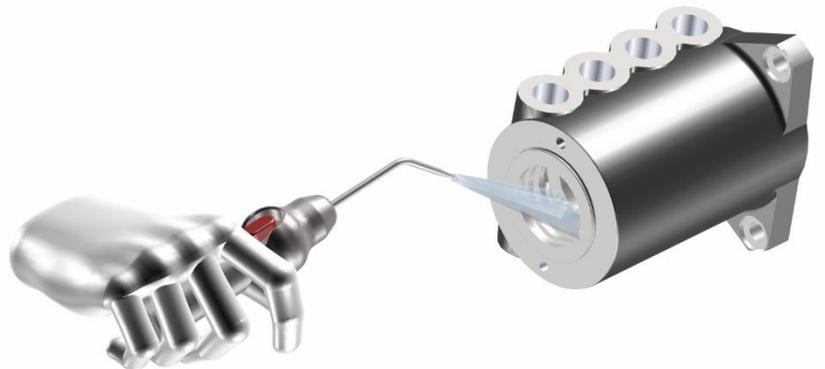
13- Place the new O-Rings "R" and the new Quad-Rings "S" in their grooves.
