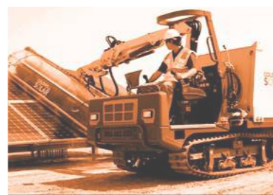
Solar Panel Cleaning
