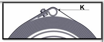
Before proceeding, check the integrity of the band "K" around the spring.
