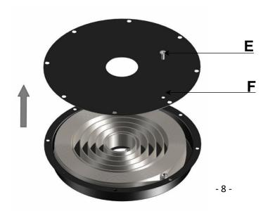
**13-** Loosen the screw "E" and lift the cover "F".
