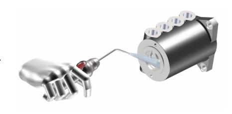
**13-** Place the new O-Rings "R" and the new Quad-Rings "S" in their grooves.
