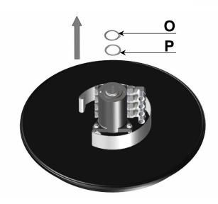
**9-** Block the shaft "Q" in a vise and unthread it as shown in the picture.
