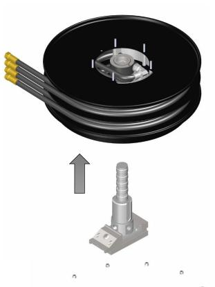
**11-** Unthread the whole reel body as shown in the picture, turn it over and place it on a workbench.
