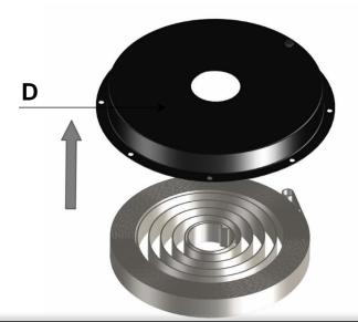
**15-** Turn over the spring container and lift the part "D".
