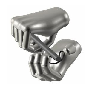
**15-** Put the deformed rings in the groove on the O-Rings and then straighten the fold by pushing it in the seat.
