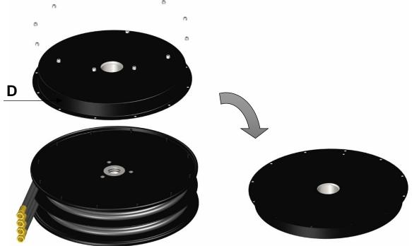
12- Lift the spring container "D" and turn it over on a bench as shown in the picture.
